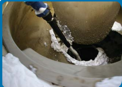
Foamhead injecting foam into truck
